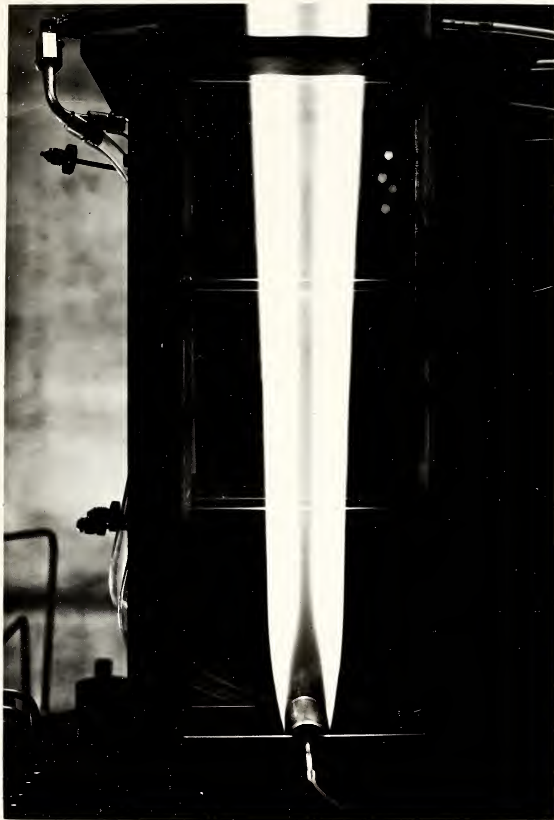
Figure 7. Time Exposure of Flame Stabilized by 1 inch Diameter Flameholder
